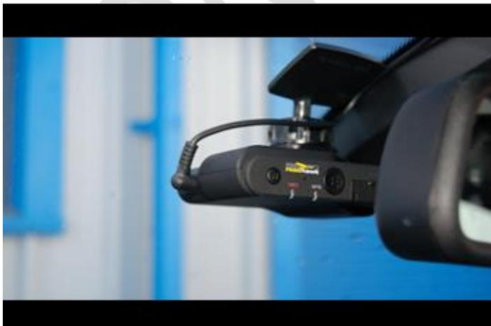
8: Plug the power cable in to the camera.
